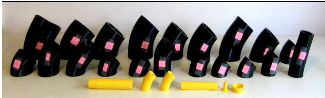
Figure 5: 3D printed Serpent parts prior to assembly
